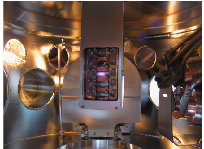
Fig. 2. Sample preparation chamber used for spin scattering experiments at the SRC. In the center are up to five sample mounts. On the right hand side is a quartz crystal oscillator (QCO) and the sample evaporators. On the left hand side is a LEED to check crystal structure.
