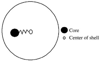
Fig. 1. Schematic of the shell model composed of a positively charged core and a massless shell with a spherical charge distribution.
