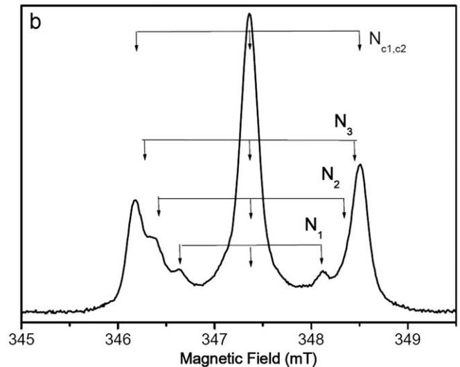
Fig. 2. D-band EPR (a) and X-band FS ESE (b) spectrum measured on highly compensated n-type 6H-SiC wafers with  $(N_D - N_A) \approx 10^{16} \text{ cm}^{-3}$  measured for  $\mathbf{B} \parallel \mathbf{c}$  at  $T = 4.2 \text{ K}$  (a) and  $\mathbf{B} \perp \mathbf{c}$  at  $T = 6 \text{ K}$  (b). Solid lines—experimental spectra, lines with symbols—simulated spectra, for parameters see Table 1.
