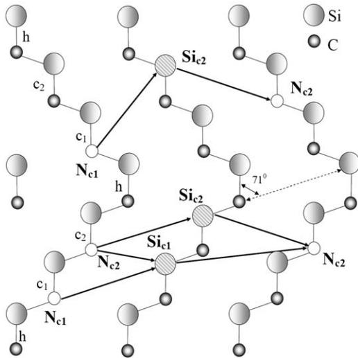
Fig. 1. Possible configurations of the distant donor pairs like  $(N_{c1}Si_{c1}N_{c1})$  on quasi-cubic lattice sites in 6H-SiC shown in the  $(11\bar{2}0)$  plane.
