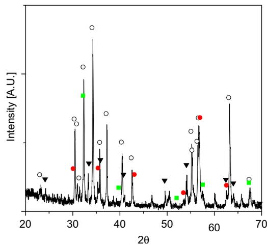
Fig. 2. X-ray diffraction pattern. Open circles:  $\text{BaFe}_{12}\text{O}_{19}$ , solid (red) circles:  $\text{CoFe}_2\text{O}_4$ , solid (black) triangles:  $\text{Fe}_2\text{O}_3$  and solid (green) squares:  $\text{LaFeO}_3$ . (For interpretation of the references to color in this figure legend, the reader is referred to the web version of this article.)
