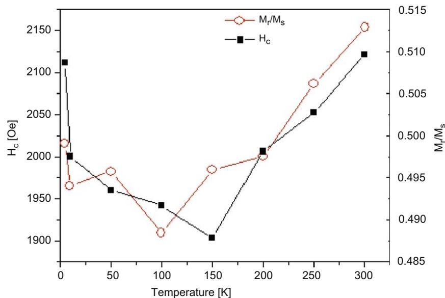
Fig. 3. Coercive field and  $M_r/M_S$  as function of temperature.
