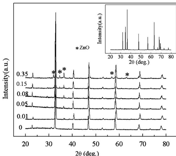
**Fig. 1.** XRD patterns for selected samples of  $(1-x)\text{LCSMO}+x(\text{ZnO})$ , with  $x = 0, 0.01, 0.05, 0.08, 0.15$  and  $0.35$ , from bottom to top; the inset shows XRD patterns for ZnO.
