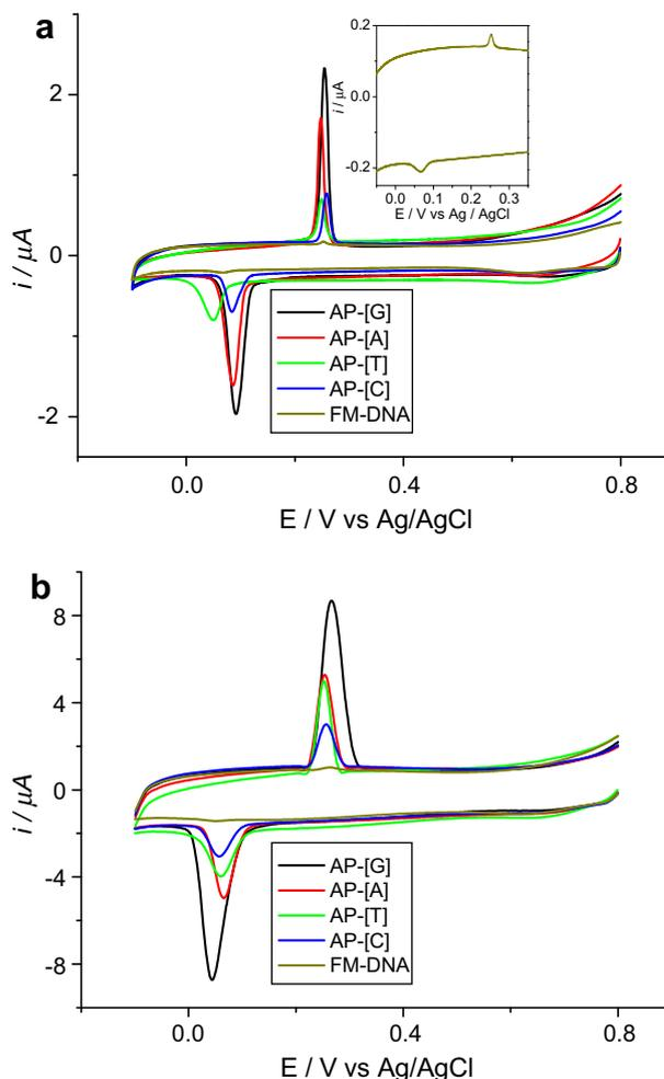
**Fig. 1.** CVs of DNA-modified gold electrodes in a 0.1 M phosphate buffer solution (pH 7.0) after 5  $\mu\text{M}$  (a) or 10  $\mu\text{M}$  (b)  $\text{AgNO}_3$  pretreatment. Inset in (a) is the CV at FM-DNA-modified electrode partially presented for displaying the small peaks. Scan rate: (a) 0.1  $\text{V s}^{-1}$ ; and (b) 1  $\text{V s}^{-1}$ .
