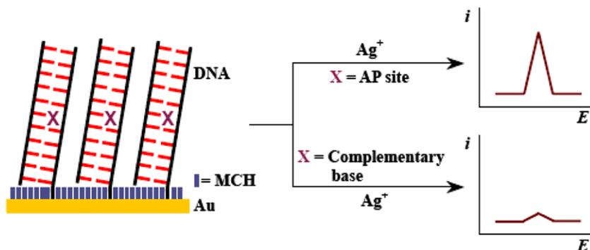
**Scheme 1.** Demonstration for construction of DNA duplex-modified gold electrode for evaluation over the binding specificity of silver cation to AP-DNA and FM-DNA.
