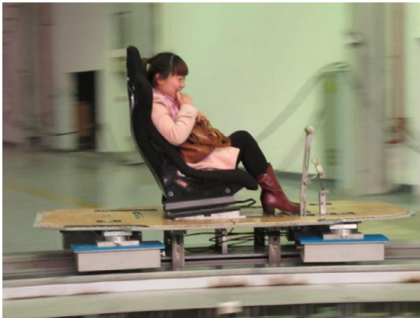
Fig. 2. The vehicle composed of four cryostats is levitating and running on a 45-m-long HTS maglev loop with a passenger.
