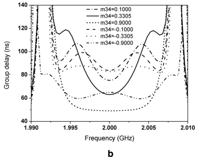
Fig. 3. The changes of group delay. (a) The group delay of Fig. 1(b) changes with  $m_{25}$ , and (b) the group delay of Fig. 1(d) changes with  $m_{34}$ .
