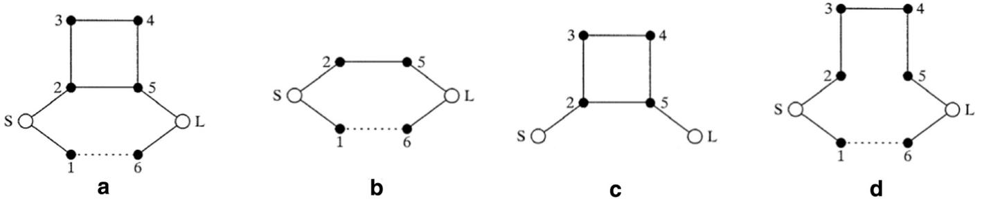
Fig. 1. The coupling and routing diagram. (a) Six-order linear phase filter, (b) Sub-network 1, (c) Sub-network 2, (d) Sub-network 3.
