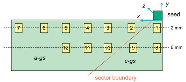
Fig. 2. Schematic drawing of the locations where the small samples were cut from the big pellet. The positions 1, 8 and 9 are located close to the seed crystal within the  $c$ -growth sector. Position 7 ( $x = 17 \text{ mm}$ ) is located outside the oriented growth sector. From all samples, we always investigated the top surface.
