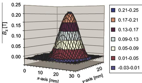
Fig. 1. Trapped field measurement of the bulk pellet before cutting. Note the homogeneous field distribution which indicates a homogeneous distribution of the flux pinning sites within the bulk pellet. A maximum trapped field of  $0.22 \text{ T}$  is recorded.
