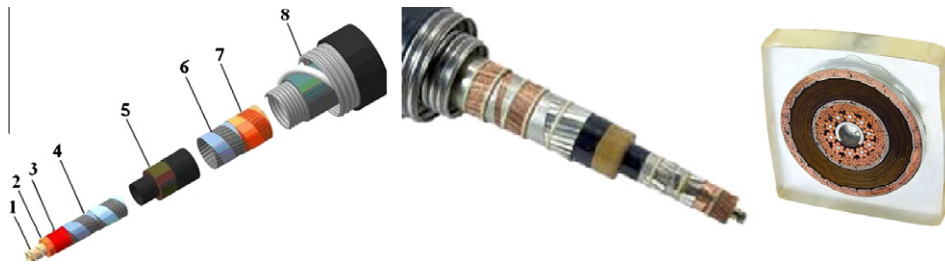
Fig. 1. Artistic view, photo of the cable model and cross-section of the phase of 200 m cable. 1 – Former – a spiral of stainless steel, surrounded by a bundle of wires made of copper and stainless steel, wrapped in copper tape – 2 and 3; 4 – two layers of HTS tapes; 5 – high-voltage paper insulation; 6 – HTS shield; 7 – flexible copper strips to protect shield, wrapped by tapes of stainless steel; 8 – flexible cryostat, 200 m long.
