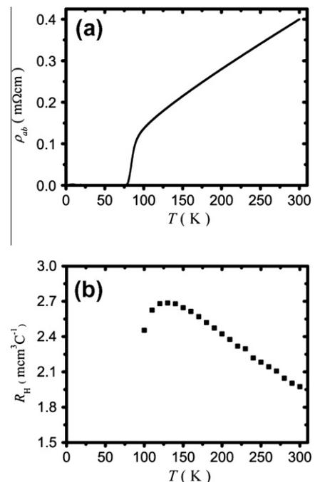
**Fig. 3.**  $T$ -dependence of the  $ab$ -plane resistivity  $\rho_{ab}$  (a) and the Hall coefficient  $R_H$  (b) for sample H-1.
