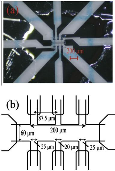
**Fig. 1.** A photograph of sample H-1 (a) and schematic illustration of the Hall-bar pattern (b).
