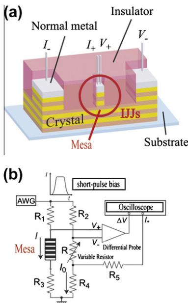
**Fig. 2.** Schematic illustration of mesa structure (a) and diagram of the circuit for short-pulse ITS (b).
