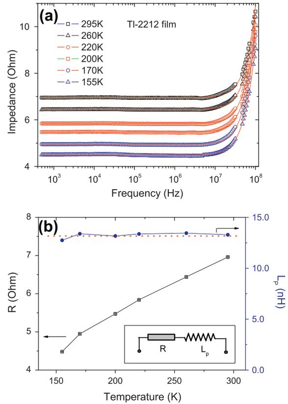
**Fig. 2.** (a) The fittings to the impedance spectrum of TI-2212 film at various temperatures in the normal states. (b) The temperature dependent resistance ( $R$ ) and parasitic inductance ( $L_p$ ). Inset: the effective circuit model used in fittings.
