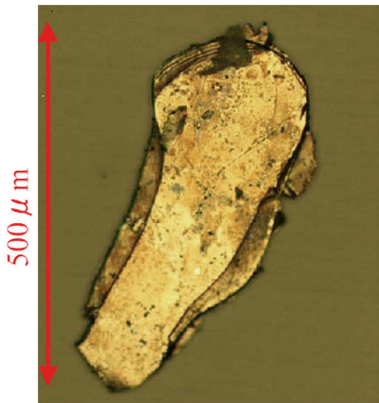
Fig. 1. Photograph of single crystal PrFeAsO 0.7 grown by high-pressure method. Length scale is presented in the arrow.
