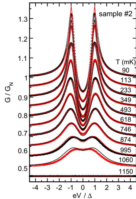
Fig. 1. Differential conductance  $G$  normalized to the normal-state value  $G_N$  for a nanostructured Al/Co point contact for different temperatures. For clarity, the curves are shifted downwards successively by 0.05 units with increasing temperature. The solid lines are calculated with the  $\tau_\uparrow - \tau_\downarrow$  model.
