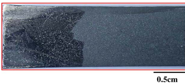
Fig. 1. Macrostructure and shape of YBCO/Ag composite fabricated by the infiltration-growth method. ( G = 26 K/cm, R = 0.18 \mu\text{m/s} ).
