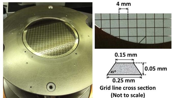
**Fig. 2.** Photo of the micro-channel plate with the calibration mask placed on top of it. The zoomed-in picture of the calibration mask and the grid line cross section are shown on the right. The diagonal line in the bottom square is to mark the orientation of the mask.
