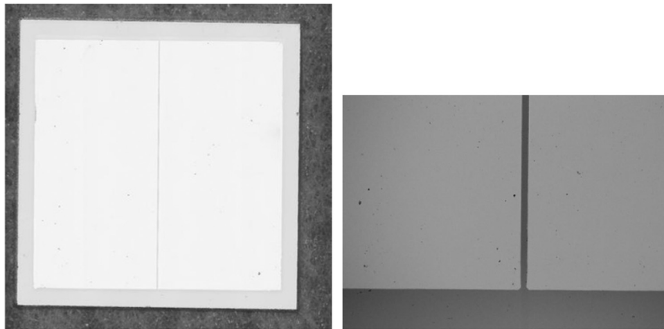
Fig. 2. A photograph of a metallized diamond sensor (left) and a zoom of the gap between the two pads (right).
