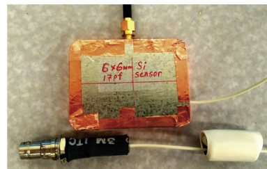
Fig. 2. The electric diagram for the silicon diode connections (left). External view of the box with silicon diode, and the bias voltage connection is shown below it (right).
