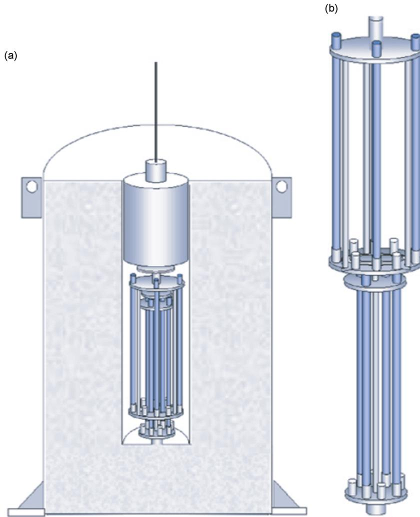
**Fig. 1.** (a) The telescopic source holder in storage position. (b) The 8  $^{60}\text{Co}$  pencils in the source holder in irradiation position.
