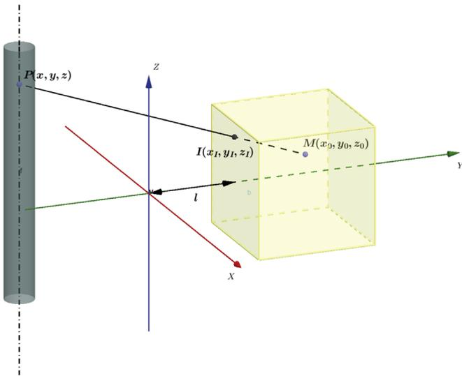
**Fig. 2.** A cylindrical source and a box shaped product in cartesian coordinates.
