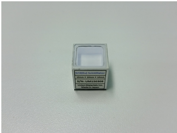
Fig. 1. Sample of cubic \text{SrI}_2(\text{Eu}) crystal encapsulated in a cubic aluminum box.
