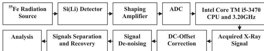
Fig. 1. Schematic diagram of the pulse height analysis of x-ray spectroscopy system.
