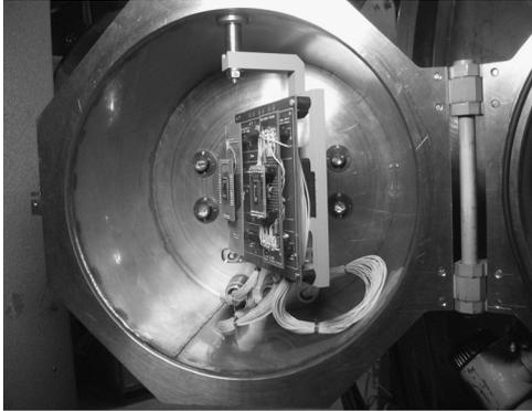
Fig. 2. Vacuum cell for mounting integrated circuits for irradiation by hard ions.
