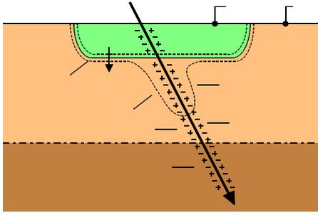
Fig. 1. Hard ion passing through a microelectronic structure [5].
