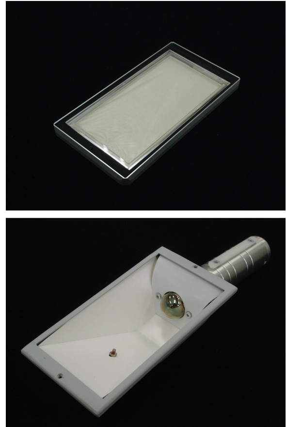
Fig. 2. Detection section of the model survey meter. (Top) Entrance window, (Bottom) light collection box with walls covered with white reflector plates. The yellow hemisphere is the PMT window. (For interpretation of the references to Colour in this figure legend, the reader is referred to the web version of this article.)
