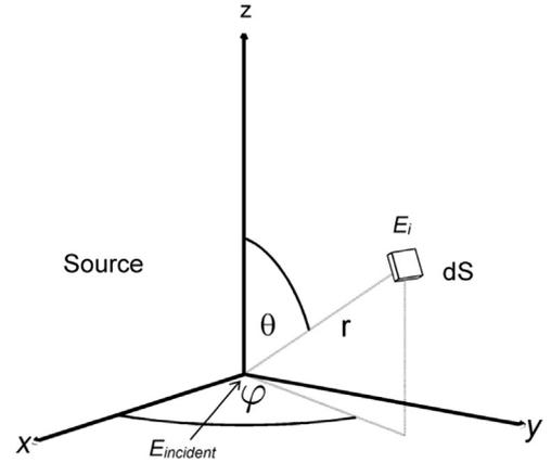
Fig. 2. Geometry for the calculation of Case A, the infinite source spectrum. A uniform isotropically-emitting alpha source is located in the +z volume. The detector plane is the x-y plane through the origin, and a point detector is located at the origin. The differential source term,  $dS$ , can be expressed as  $dS = s_v r^2 dr d\Omega$ , where  $dr$  is the differential distance in the direction of  $r$  and  $d\Omega$  is the differential solid angle.
