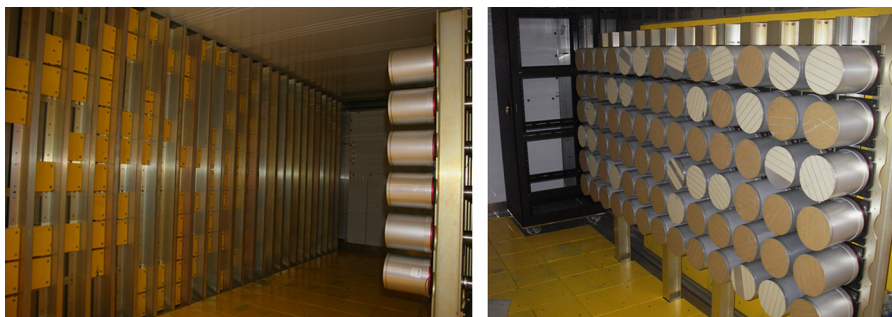
Fig. 2. A view from inside the container shows the \gamma -ray, coded-aperture imaging system. Upon entering, the left side of the container comprises the array of lead coded-mask elements ( 10 \text{ cm} \times 10 \text{ cm} \times 5 \text{ cm} ) mounted to the inner container wall. The opposite facing side of the container comprises the 6 \times 13 array of 12.7 cm NaI(Tl) detectors. Adjacent to the detector array are the associated VME and NIM electronics and power supply.
