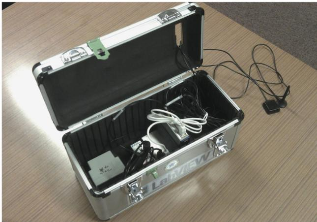
**Fig. 2.** In-vehicle part of KURAMA-II. The components are placed in a small tool box (34.5 cm × 17.5 cm × 19.5 cm) for the better handling. This tool box is made of 1 cm thick balsa wood plates covered with thin aluminum sheets, and no effective shielding towards typical  $\gamma$ -rays in environment.
