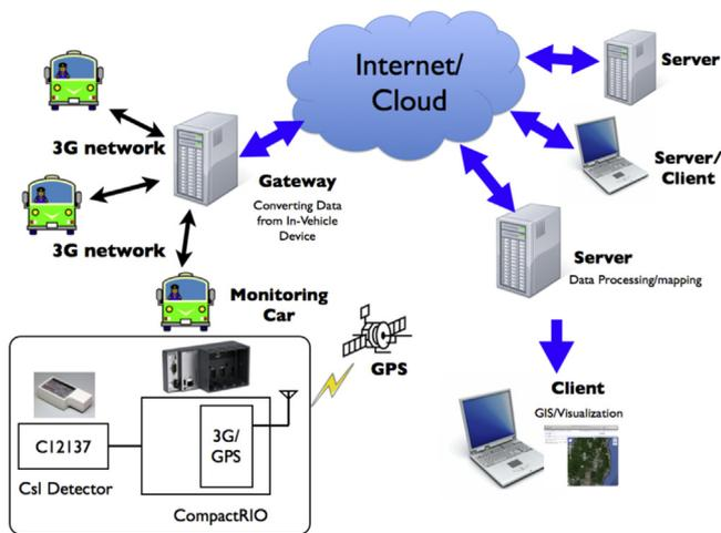
**Fig. 1.** System outline of KURAMA-II. The scheme is basically the same as that of KURAMA, but a gateway server is introduced for the conversion of data chunks from in-vehicle units to data files shared over Dropbox [5] due to no support of Dropbox on CompactRIO.
