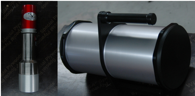
Fig. 1. Borated plastic scintillator (76 mm × 76 mm) coupled to a photomultiplier and a digital MCA (left). Detector in the final lead shield package (right). The lead shield covers the scintillator and is 23 mm thick on the side, 10 mm thick in the front, and extends 5.4 cm behind the scintillator.
