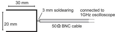
**Fig. 2.** Configuration of Faraday cup. Beams are mainly captured at the bottom of the FC.
