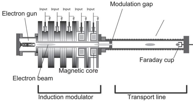
**Fig. 1.** Schematic diagram of the device for bunching experiment. Injected electrons are manipulated by modulation voltage and longitudinally compressed in the transport line.
