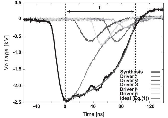
**Fig. 3.** Modulation voltage for longitudinal compression. Sharp gray line shows ideal waveform defined by Eq. (1) for  $L_f = 1.942$  m, and bold black line denotes synthesized waveform with induction adder.
