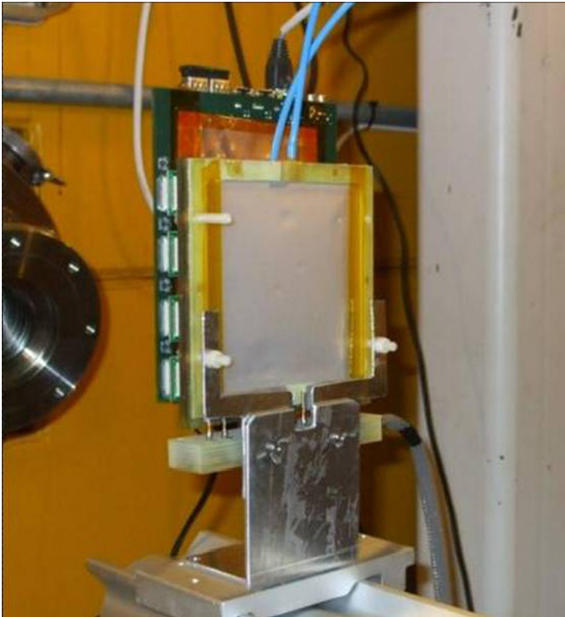
Fig. 1. Front view of the nGEM detector installed on the Vesuvio beam line.
