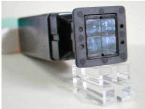
Fig. 3. Light guides and polycarbonate support.
