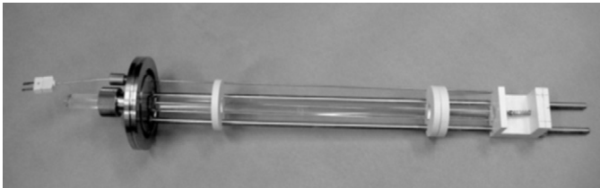
Fig. 2. View of the scintillator sample holder assembly. The white rings are boron nitride (BN) spacers used to center and align the insert in the stainless steel enclosure. The white sample holder assembly located near the end of the two stainless steel support rods consists of a BN body with a moveable spring-loaded platen that holds the scintillator sample flat against the end of the quartz light guide.
