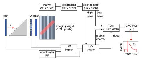
Fig. 2. Block diagram of the readout, trigger and data acquisition chain of FAST.
