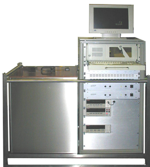
Fig. 1. Photo of the small sample calorimeter.
