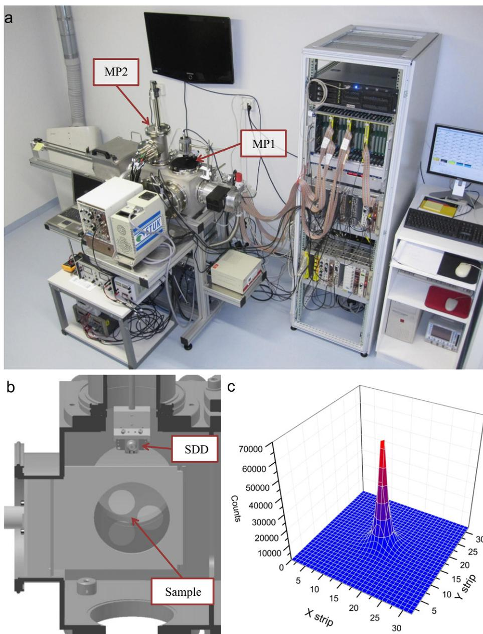
**Fig. 1.** Upgraded PANDA setup. (a) Photograph of the setup (b) Technical drawing showing MP2. The samples are transported between the measurement positions using a horizontally moving linear feedthrough and the SDD detector is moved with a vertically moving linear feedthrough. (c) Alpha particle hitmap of a  $^{241}\text{Am}$  sample measured using the position sensitive DSSSD in MP1. The hitmap information can be used to set the interesting part of the sample to directly face the SDD.
