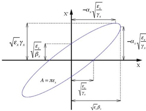
**Fig. 2.** The Courant Snyder ellipse and the relevant geometrical interpretation.
