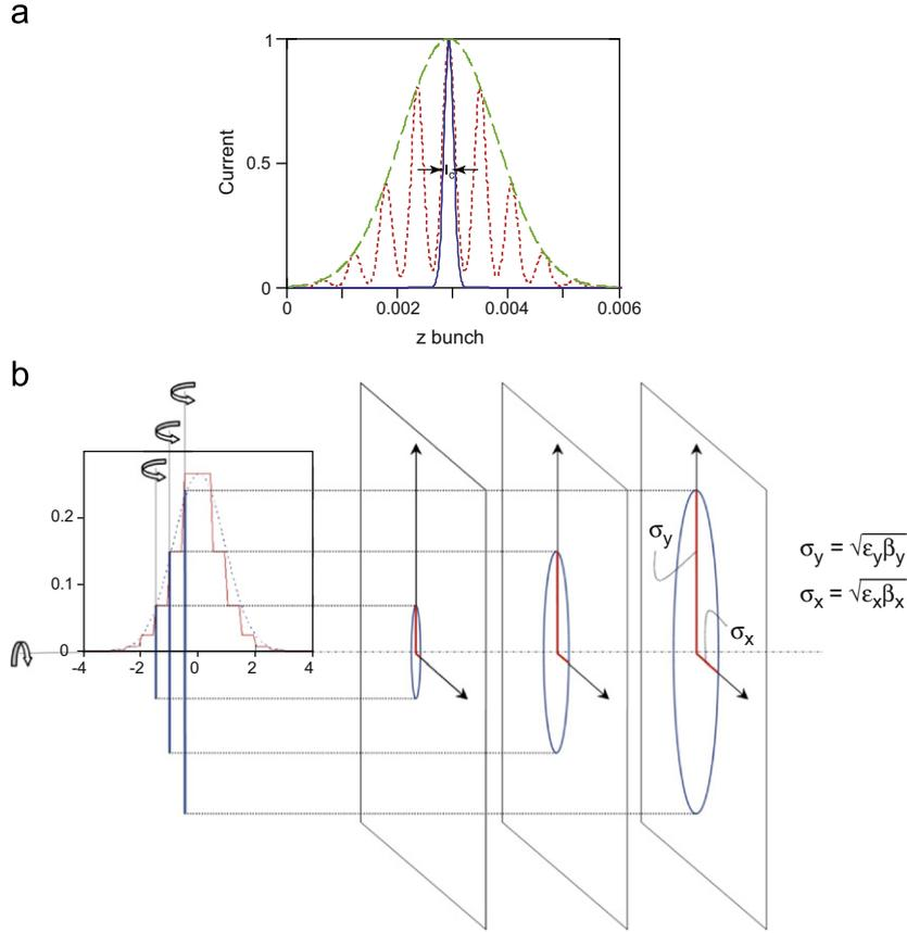
**Fig. 1.** (a) Local interaction and slice emittance, the dash line is the bunch envelope, the dot line represents the slices and the continuous line is the radiation distribution associated with the slice,  $l_c$  being the coherent length; (b) transverse sections of the sliced bunch.
