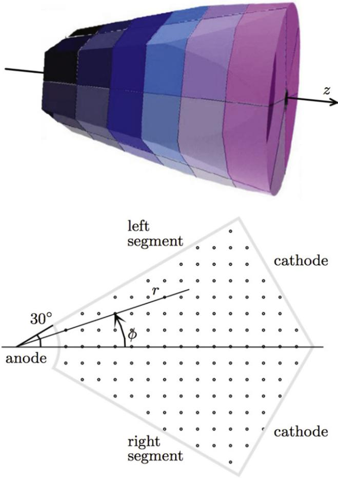
**Fig. 1.** (Color online). Upper panel: AGATA HPGe crystal. The outer surface is covered by 36 cathodes (six rings of six portions). A central hole along the z-axis is covered by the anode. The length of the crystal is 90 mm and its maximum diameter is 80 mm. Lower panel: typical segment as seen perpendicular to the z-axis. The dots show the locations of the simulated hits for a  $2 \times 2 \times 2$  mm grid.
