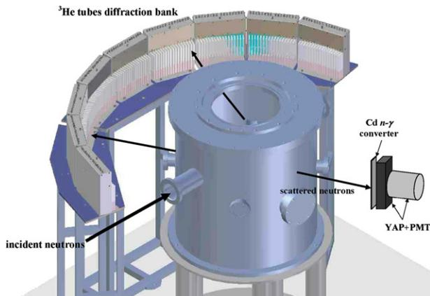
Fig. 1. Schematic layout of the INES powder diffraction diffractometer at ISIS during the experiment. The instrument was equipped with the new YAP–Cd device for non-standard diffraction measurements.
