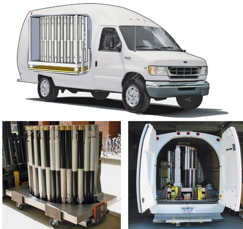
Fig. 1. SORIS system (lower left) before installation in the van and (lower right) after installation. Top is a rendition showing the system's relative placement after installation.
