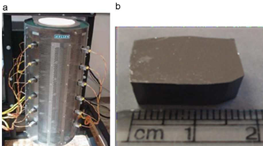
Fig. 1. Modified vertical Bridgman furnace (a) used to grow BiI<sub>3</sub> crystals (b).
