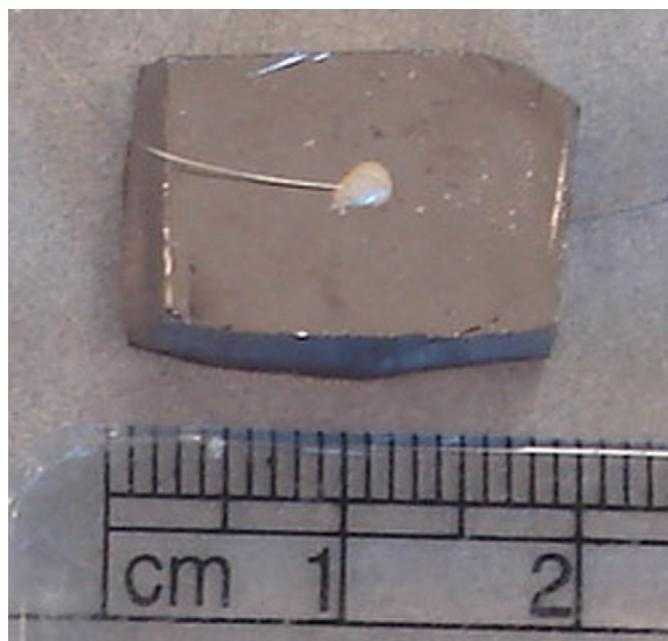
Fig. 3. Detector fabricated with Pd electrodes.
