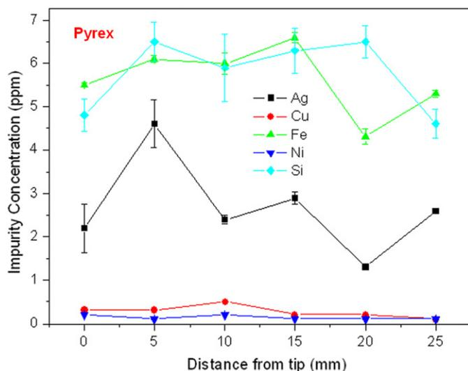
Fig. 2. Impurity analysis performed along the length of the crystal.
