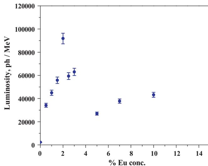
Fig. 2. Eu concentration dependence scintillation light yield of  $\text{CsBa}_2\text{Br}_5:\text{Eu}$ .
