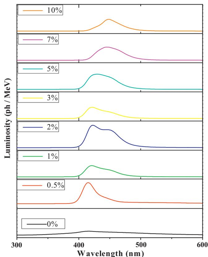
Fig. 1. X-ray excited emission spectra of undoped and an Eu doped  $\text{CsBa}_2\text{Br}_5$ . Inset figures indicate %Eu concentration.
