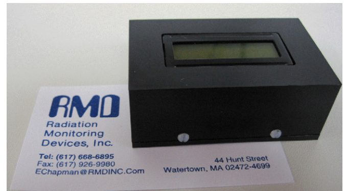
Fig. 5. Photograph of charged particle dosimeter module on a business card to provide scale. The module contains a battery, power supply circuitry, amplifier, a peak hold circuit and a microprocessor, which digitizes and stores the pulse heights. A USB connection provides battery connection and data readout.
