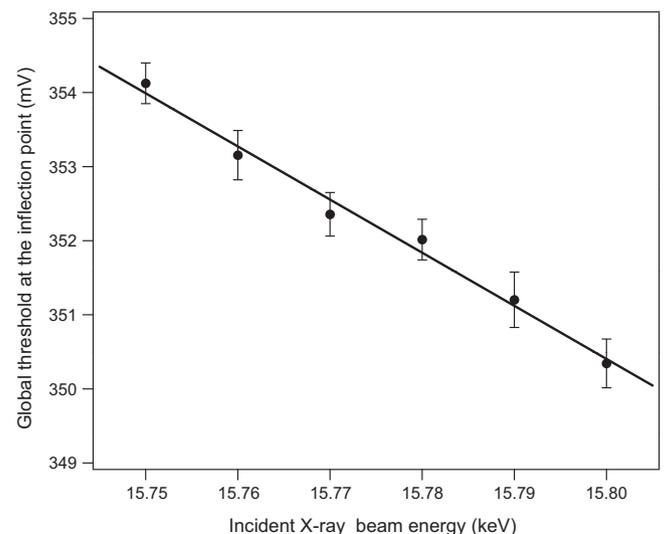
Fig. 2. Estimated threshold voltages at the inflection points for 15.75, 15.76, 15.77, 15.78, 15.79, and 15.80 keV X-ray beams.
