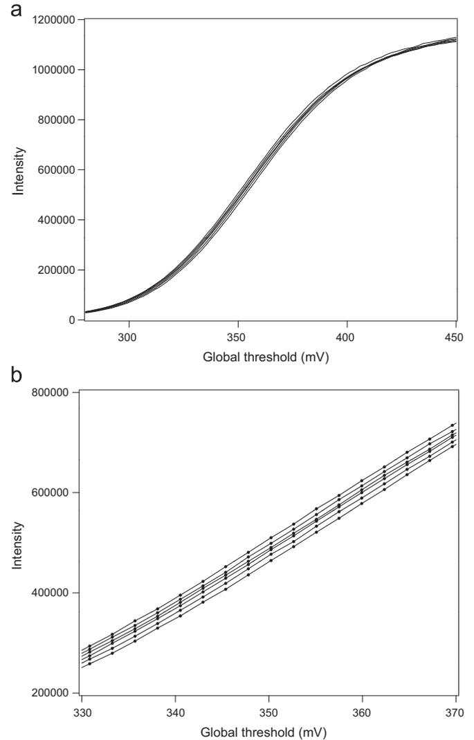
Fig. 1. (a) Global threshold scans for 15.75, 15.76, 15.77, 15.78, 15.79, and 15.80 keV X-ray beams. (b) Global threshold scans around the inflection points for 15.75, 15.76, 15.77, 15.78, 15.79, and 15.80 keV X-ray beams.
