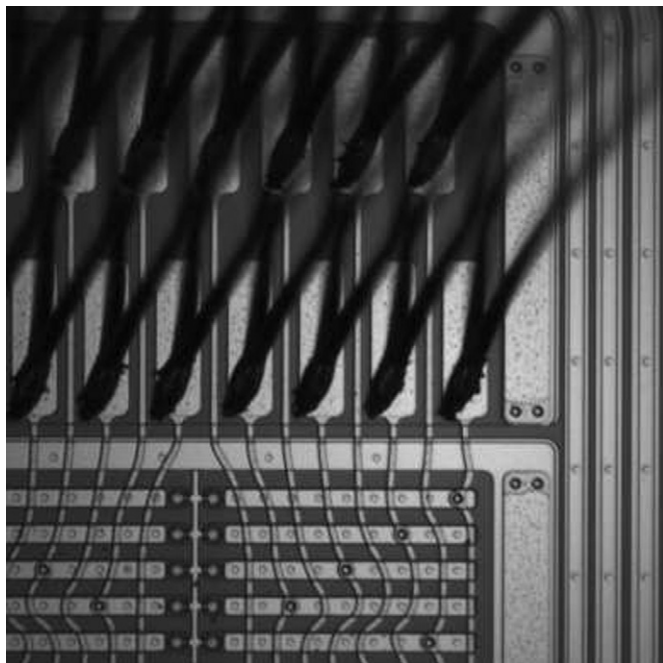
Fig. 1. Sensor with interleaved readout pixels. Second metal layer provides their interconnect and routing to the wire bond pad. Shuffling of readout channels minimises their cross-talk.
