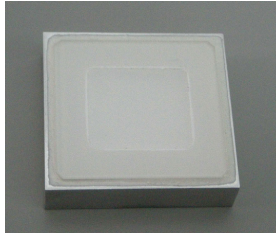
Fig. 1. Continuous \text{LaBr}_3 crystal surrounded by reflective material and encapsulated in an aluminum housing.
