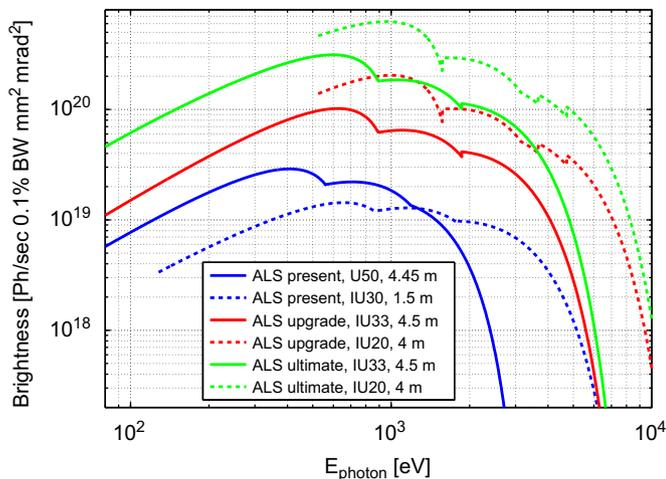
**Fig. 1.** Comparison of the current ALS brightness around 1 keV (i.e. after top-off upgrade) with future brightness after the low emittance upgrade (as well as a more speculative case, if low horizontal beta function lattices are workable).
