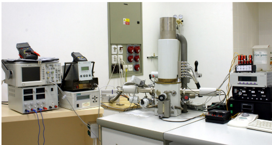
Fig. 1. Non-commercial experimental scanning electron microscope AQUASEM-II.
