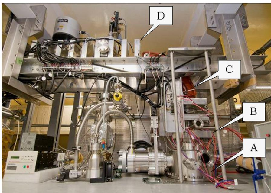
**Fig. 1.** An overview of the brightness enhancer and the end of the beam line. (A) Brightness enhancer. (B) Final Helmholtz coil. (C)  $90^\circ$  bending solenoid. (D) Helmholtz coils.
