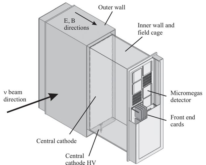
**Fig. 1.** Simplified cut-away drawing showing the main aspects of the TPC design. The ND280 off-axis detector uses a right handed coordinate system with  $z$  in the horizontal plane along the neutrino beam direction, and  $y$  in the vertical direction.
