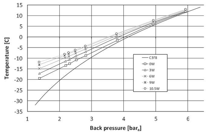
**Fig. 2.** Measured evaporation temperature as a function of the back pressure for different detector power. For comparison the saturation curve for  $C_3F_8$  is shown.
