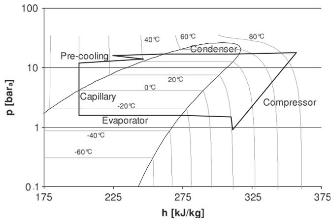
**Fig. 1.** Phase diagram for  $C_3F_8$  and design thermodynamic cycle of the ATLAS Inner Detector evaporative cooling system.
