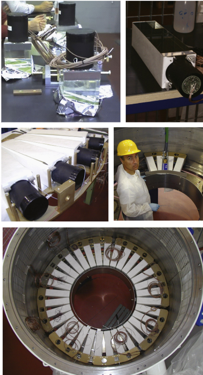
Fig. 2. LAV station assembly phases (from top-left): cabling of PMT, wrapping of crystals, mounting of four-crystals brackets, fixing of brackets inside the steel cylinder, routing of cables to vacuum flange ports.
